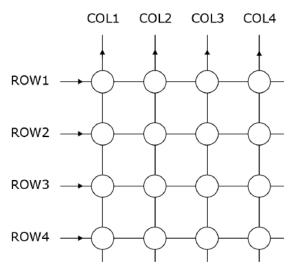
The buttons are connected in a  $4 \times 4$  matrix to the ROW1-4 (output) and COL1-4 (inputs) terminals. If you do not make use of all of the 16 buttons, you can leave some of the ROW and COL signals unconnected. If you need one button only, connect it to the ROW1 and COL4 terminals.
